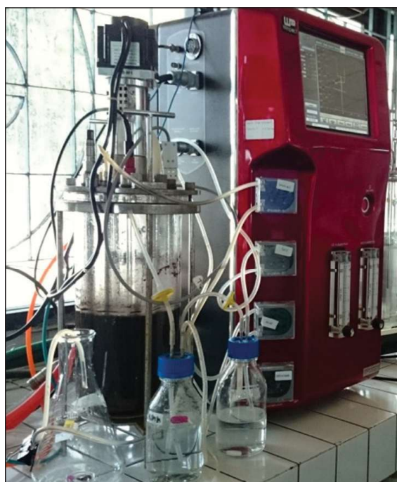
Figure 1. Fermentor MBI Winpact One Fermentation System for biomasses fermentation.
